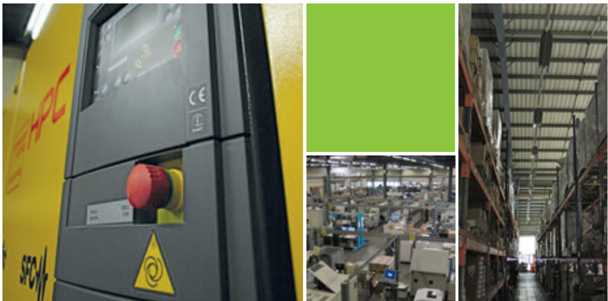
Efficient variable speed compressor with heat exchanger, which also saves on space heating bills.
